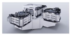
The TRUMPF laser amplifier, a pulse-type CO2 laser system, delivers the laser pulse for the EUV project.
