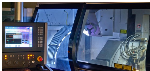
With the TruLaser Tube 7000 the tube specialists of ProfilLaseRichter have opportunities that many customers don't even know, yet. Examples are bending connections and also positioning aids with locating pins and cut-outs to simplify assembly. Thanks to the degree of automation in the machine the throughput times are shorter and so are the delivery times. Picture: Escherich Fotografie
