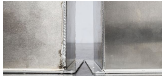
Werner Neumann’s expectations in regard to the reduction in retouching work were satisfied completely by laser welding. For some parts the touch-up time could be reduced from twelve hours to just 90 minutes.
