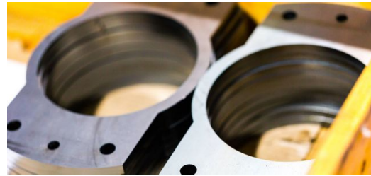
Thomas Sattler: "The relationship of bore diameter to sheet thickness is fantastic, and we can mostly do away with the extra milling we had to do in the past." (Picture: Thomas Abé)
