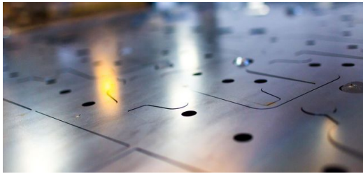
CoolLine is a function that enables targeted workpiece cooling and thus to nest components much more tightly than before. (Picture: Thomas Abé)
