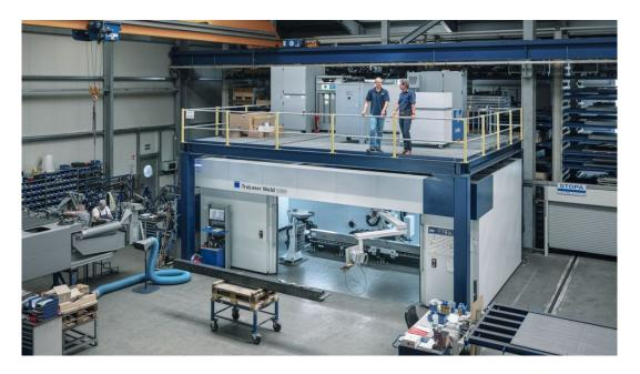
To save space, all the TruLaser Weld 5000's peripherals and system technology are positioned on a dedicated enclosure above the machine. © Günther Bayerl
