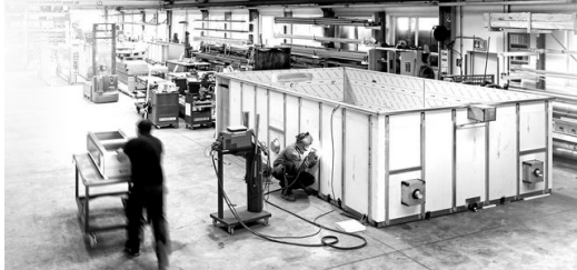
In one piece: Pools with standard dimensions are fully finished at Gassner and transported to the installation site on flatbed trucks. Picture: Niels Schubert
