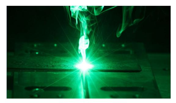
Using green light, copper welding becomes more energy efficient and of higher quality, irrespective of the properties of the material surface.
