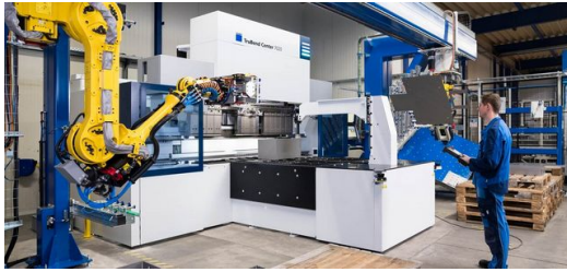
The new TruBend Center 7020 panel bender made production of the field stove possible in the first place. Only with this equipment was the team at Kuipers able to automatically bend the relatively large firebox of 333 millimeters.
