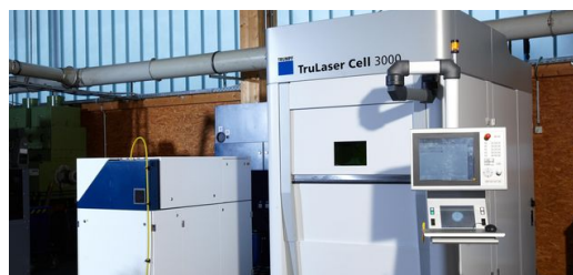
"The quality of the edge produced with the solid-state laser, even when cutting thicker materials, is just as good as with the CO 2 laser," Franz Biegert emphasizes. Picture: Florian Bilger Fotodesign
